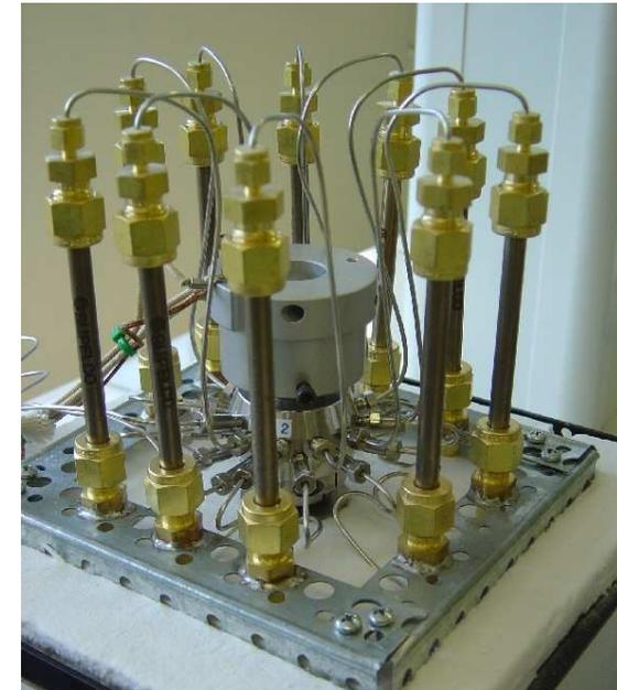
**SPA tubes coupled to a multiport valve for fast sampling (> 2 sec.)**
